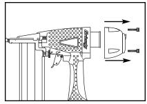
Figure 7. Removing rear cap.
